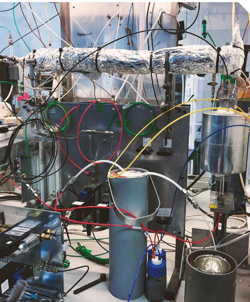
LABORATORY PLANT FOR THE PRODUCTION OF CNTS IN ST. ANDREWS
